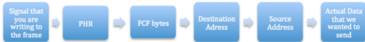
FIGURE 3: Procedure to Send a Data Packet
